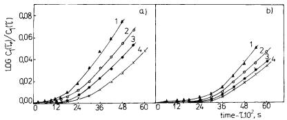
Fig. 1. Log  $C_1(\tau_0)/C_1(\tau)$  vs. time for sodium chloride transport across the membranes at different toluene (a) and heptane (b) content in the monomer mixture: (1) 5 wt %; (2) 10 wt %; (3) 20 wt %; (4) 30 wt %. The DVB content is 3 wt %.
